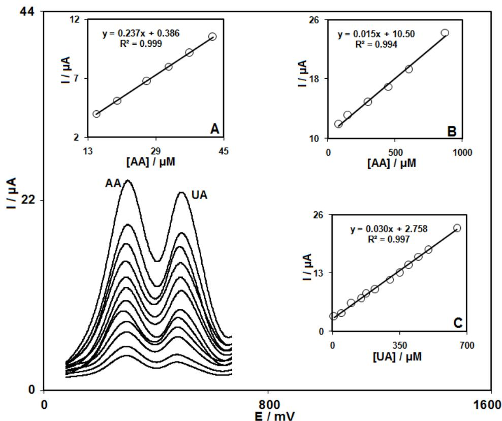
Fig. 6. DPVs of MC-CNPE in 0.1 M PBS (pH 7.0) containing different concentrations of AA+UA in  $\mu\text{M}$ , from inner to outer: 15.0+10.0, 20.0+50.0, 27.0+100.0, 32.0+150.0, 37.0+175.0, 42.5+225.0, 80.0+300.0, 150.0+350.0, 300.0+400.0, 450.0+450.0, 600.0+500.0, and 875.0+650.0 respectively. Insets (A), (B) and (C) are plots of  $I_p$  vs. AA and UA concentrations, respectively.
