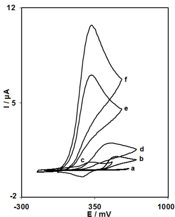
Fig. 3. CVs of (a) unmodified CPE in 0.1 M PBS (pH 7.0) at scan rate of  $10 \text{ mV s}^{-1}$ ; (b) as (a) + 0.1 mM AA; (c) as (a) at the surface of MC-CNPE; (d) as (b) at the surface of CNPE; (e) as (b) at the surface of MC-CPE; (f) as (b) at the surface of MC-CNPE.
