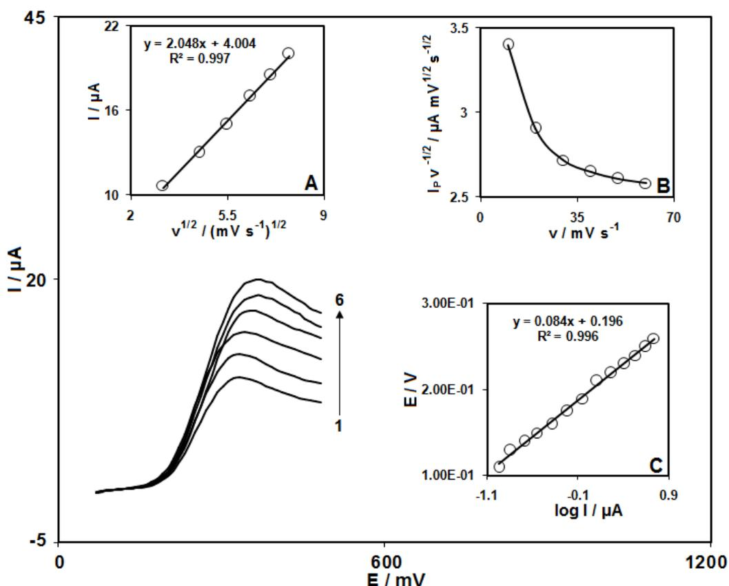
Fig. 4. Linear sweep voltammograms of MC-CNPE in 0.1 M PBS (pH 7.0) containing 100.0  $\mu\text{M}$  AA at various scan rates; From inner to outer scan rates of 10, 20, 30, 40, 50 and 60  $\text{mV s}^{-1}$ , respectively. Insets: variation of (A) anodic peak current vs.  $v^{1/2}$ ; (B) normalized current ( $I_p/v^{1/2}$ ) vs.  $v$ ; (C) Tafel plot derived from the rising part of the voltammograms recorded at the scan rates of 10  $\text{mV s}^{-1}$ .
