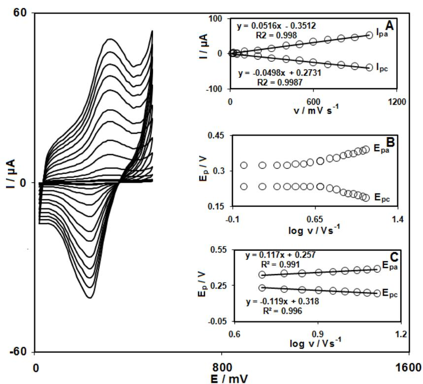
Fig. 2. CVs of MC-CNPE in 0.1 M PBS (pH 7.0), at various scan rates, from inner to outer, 10, 20, 50, 100, 200, 300, 400, 500, 600, 700, 800, 900 and 1000  $\text{mV s}^{-1}$ . Insets: (A) Variations of  $I_p$  versus different scan rates: 10, 20, 50, 100, 200, 300, 400, 500, 600, 700, 800, 900 and 1000  $\text{mV}^{-1}$ . (B) Variation of  $E_p$  vs. the logarithm of scan rates; (C) Variation of  $E_p$  versus the logarithm of the high scan rates.
